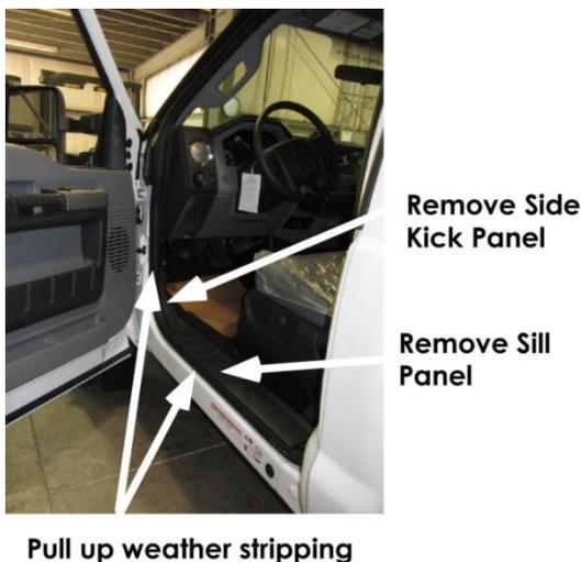
**Figure 1. Accessing inside of side kick panel.**
