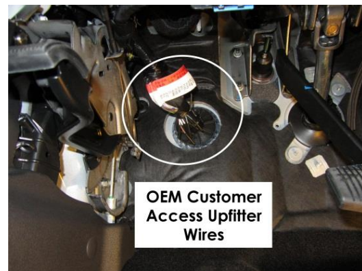
Figure 3. Customer Access wires.
