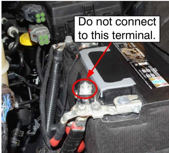
Figure 54. OEM Upfitter Driver Side Terminal Connection instruction.
