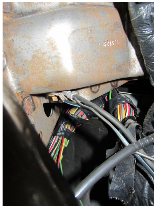
Figure 46. Firewall ground stud—driver side under dash
