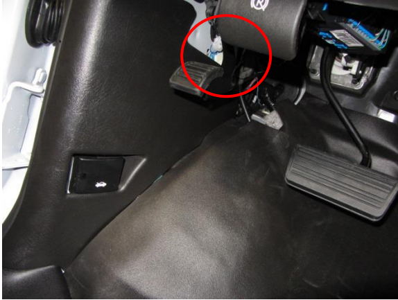
Figure 63. CAN connector recommended location.
