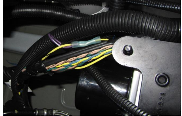
Figure 65. Splicing LS Purple/White wire to OEM Yellow/Black wire.
