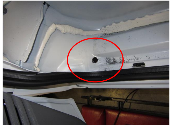
Figure 57. Access hole drilled into driver side foot well.
