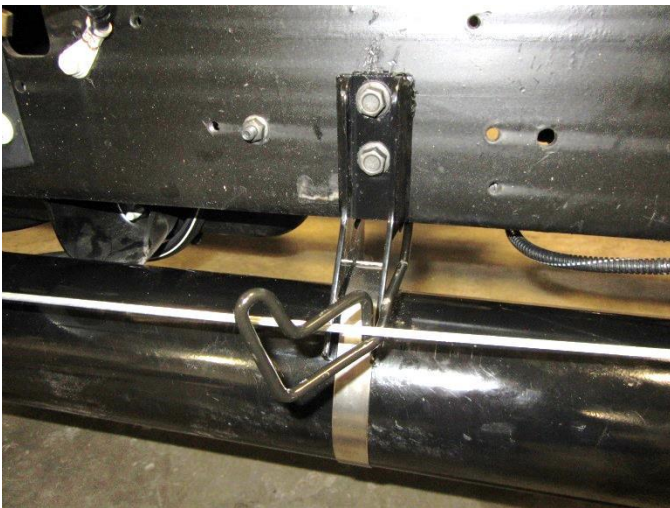
Figure 46. Reshape wire keeper to hold parking brake cable away from volume mounts.
