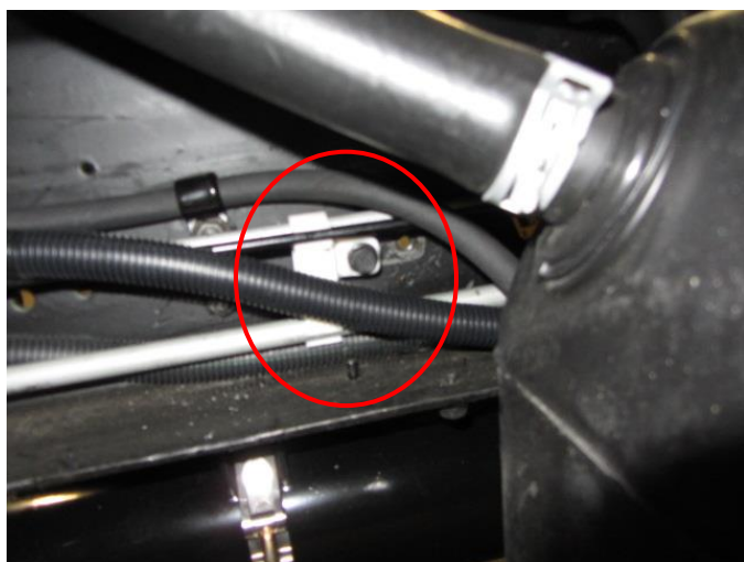
Figure 42. Fuel line clip spaced away from frame.
