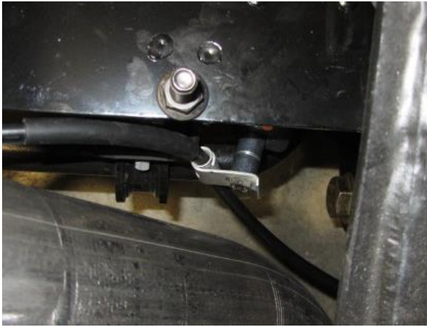
Figure 45. Passenger side parking brake remounting.
