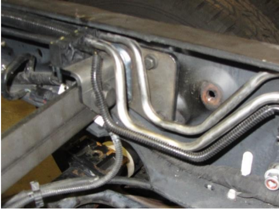
Figure 17 Fuel Lines route over top of Tie Bar Mount
