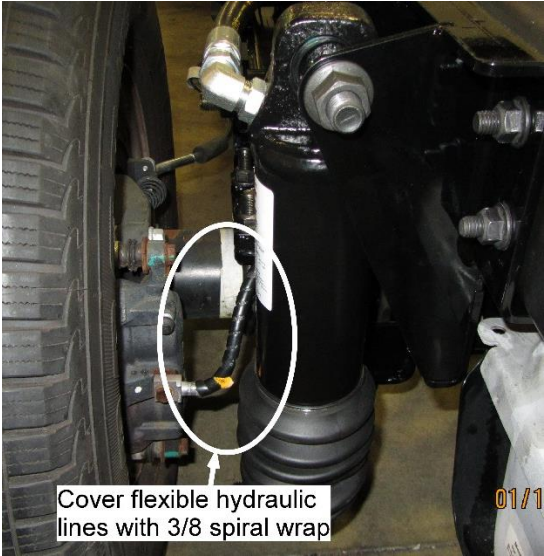
Figure 19: Install spiral wrap around brake whip hoses, on Driver and Passenger sides
