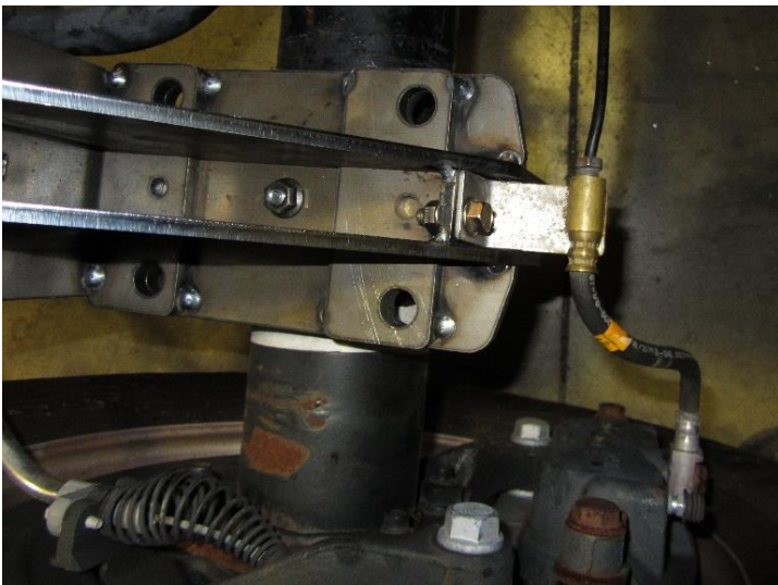
Figure 9. Attachment of driver side brake flexible line.
