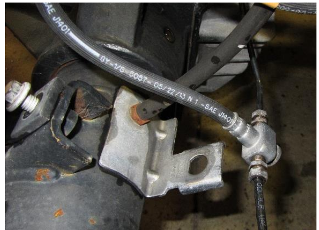
Figure 8. Middle Tee bracket to remove.
