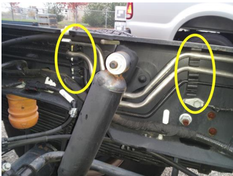
Figure 15. Fuel and Brake Line Retainers to disconnect
