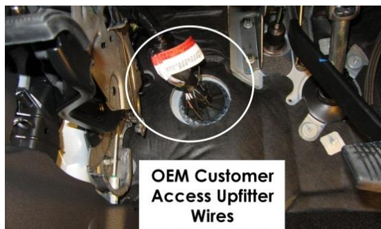
Figure 30. Customer Access wires.
