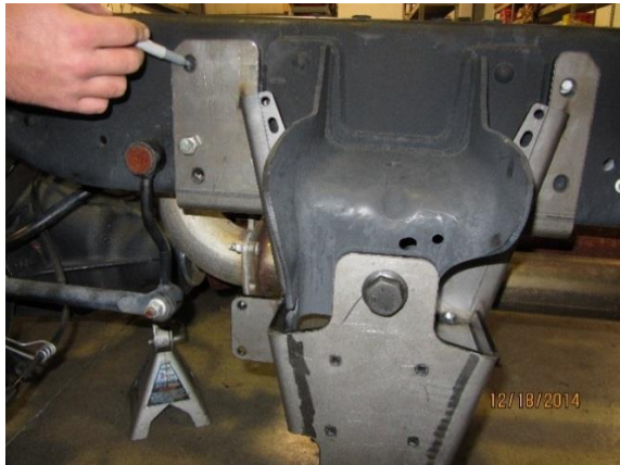
Figure 6: Passenger side hanger shown, marking holes for drilling
