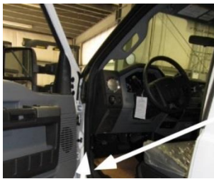
Figure 28. Accessing inside of side kick panel.
