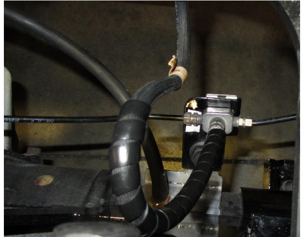
Figure 11: Top-Down view of Rear Brake Splitter
