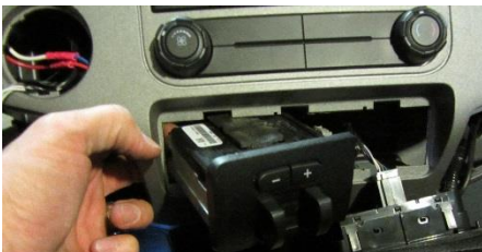
Figure 34: Trailer Brake Module in Dash
