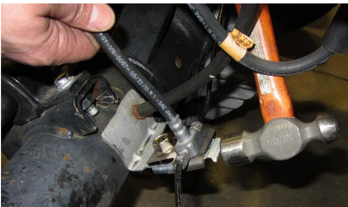
Figure 10. Attachment of relocation plate to splitter tee.
