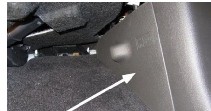
Figure 37. Passenger side kick panel to remove.
