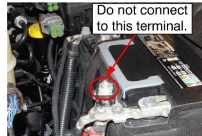
Figure 27. OEM Upfitter Driver Side Terminal Connection instruction.
