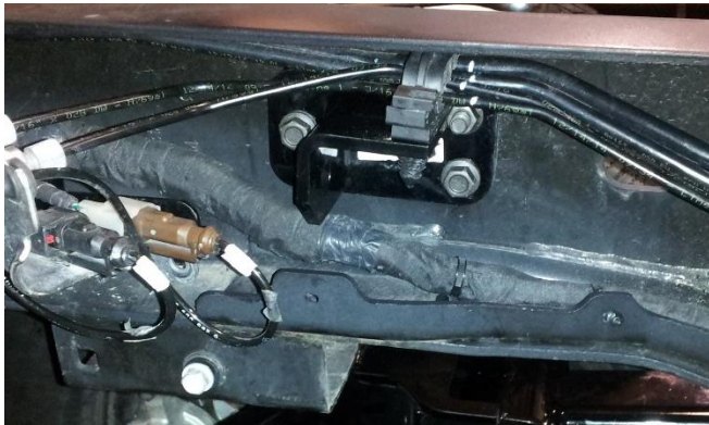
Figure 12: Tie Plate Bracket installed with fuel and brake lines reattached
