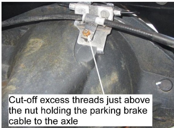
Figure 10: Trim Stud to allow clearance in full Jounce
