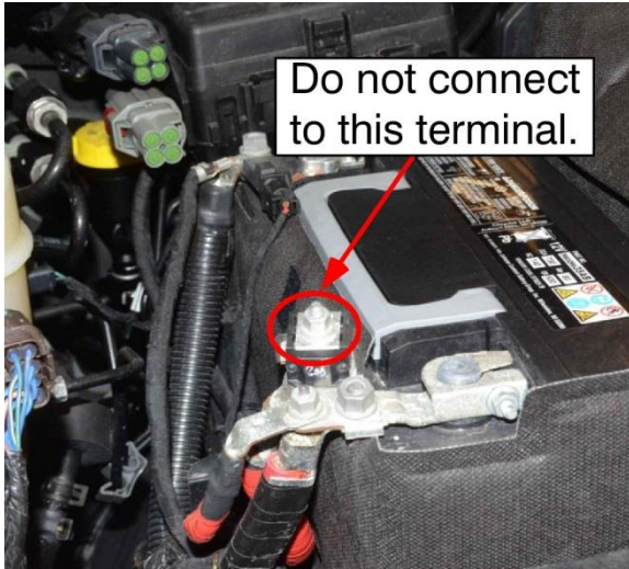
Figure 27. OEM Upfitter Driver Side Terminal Connection instruction.
