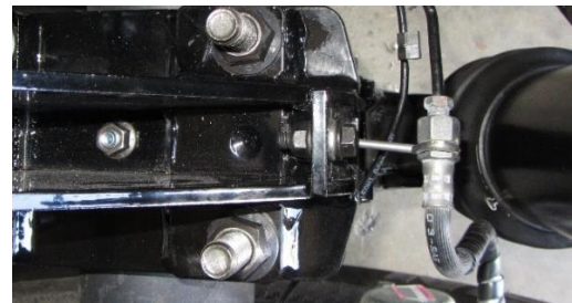
Figure 8. Attachment of driver side brake flexible line.
