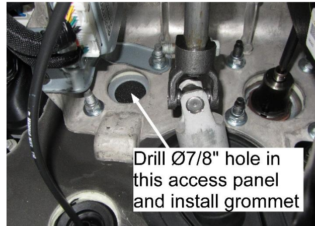
Figure 25: Cover plate to route harness through
