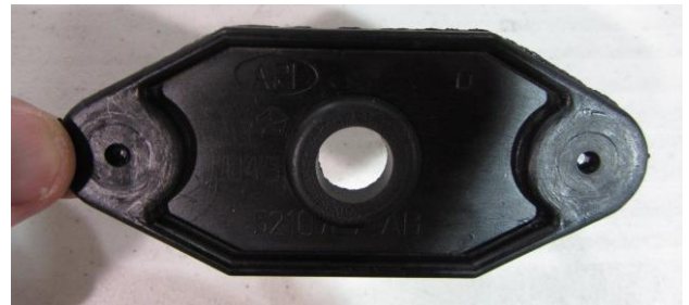
Figure 26. Modified Clutch Linkage Cover Plate (Removed from vehicle)
