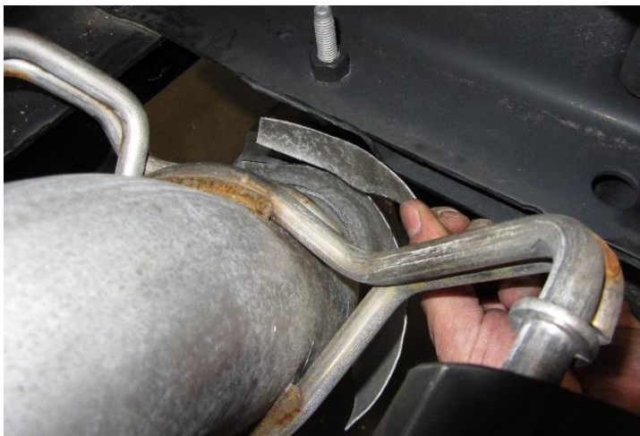
Figure 6: Material to remove from Heat Shield
