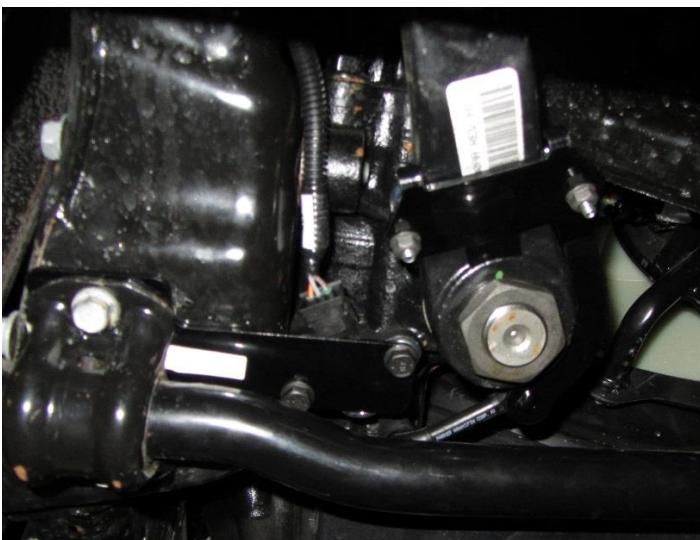
Figure 19. Sensor mount installs above the swaybar.
