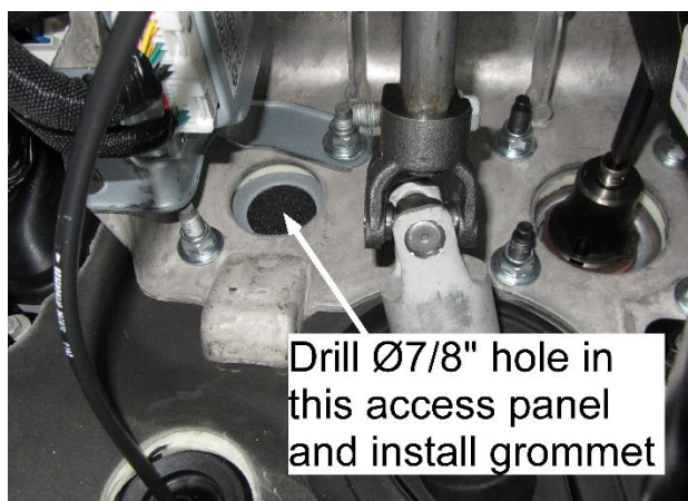
Figure 44: Cover plate to route harness through
