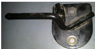
Figure 8: Enlarge holes to Ø17/32"
