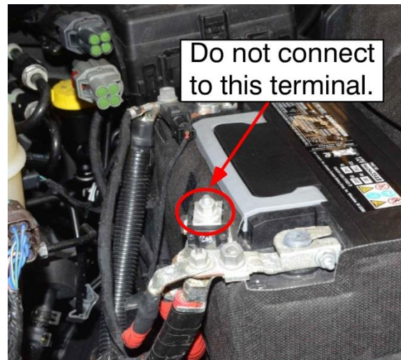
Figure 46. OEM Upfitter Driver Side Terminal Connection instruction.
