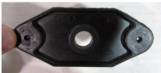
Figure 45. Modified Cover Plate (Removed from vehicle)
