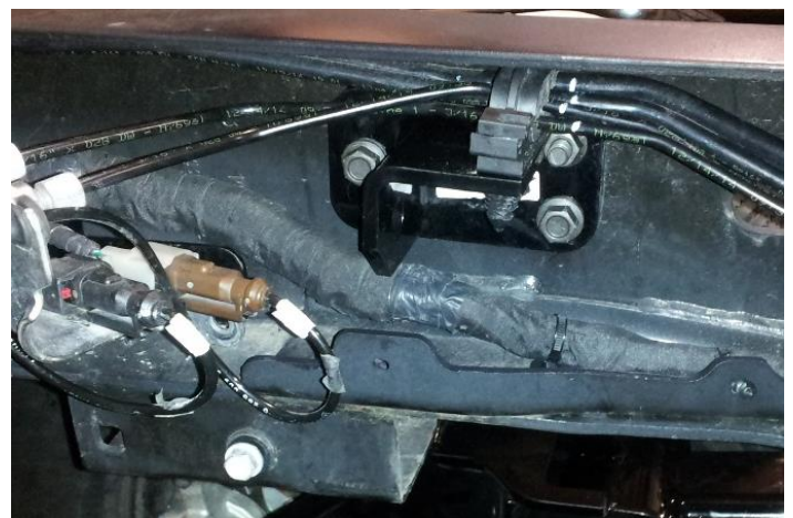
Figure 13: Tie Plate Bracket installed with fuel and brake lines reattached
