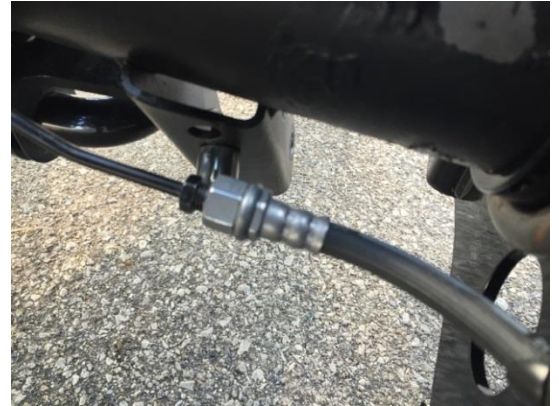
Figure 16. Use spacer and M8 bolt to re-attach bracket
