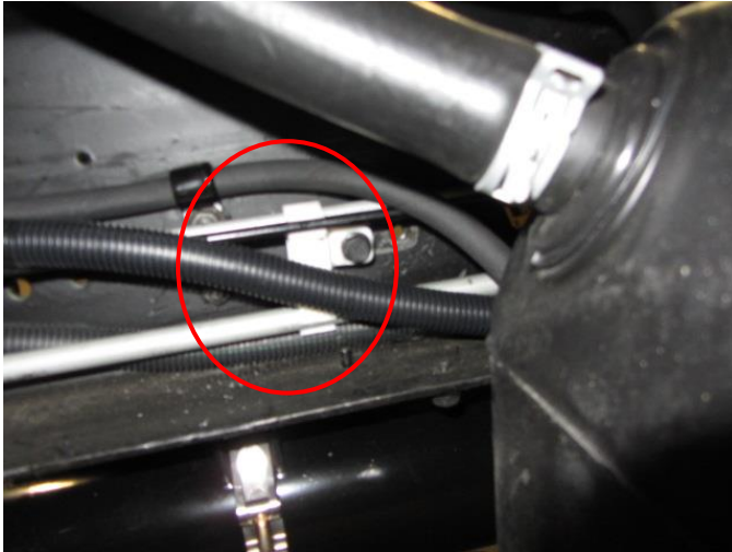
Figure 55. Fuel line clip spaced away from frame.
