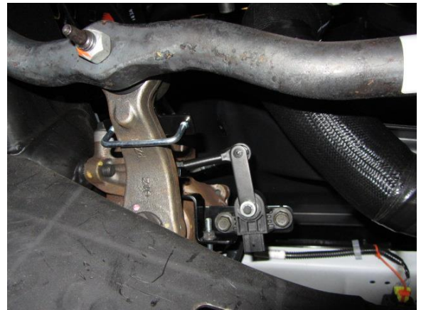
Figure 67. Steering sensor components installed.
