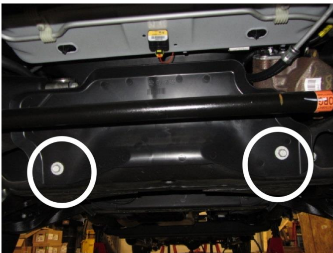
Figure 63. Access panel removal.
