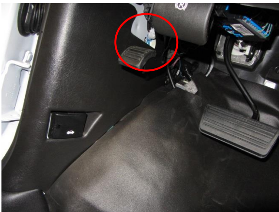
Figure 75. CAN connector recommended location.
