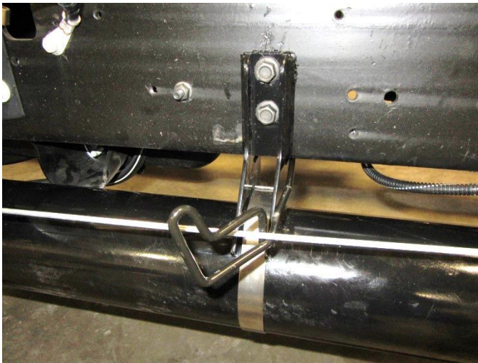
Figure 59. Reshape wire keeper to hold parking brake cable away from volume mounts.
