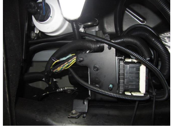
Figure 76. ABS actuator, under cab.
