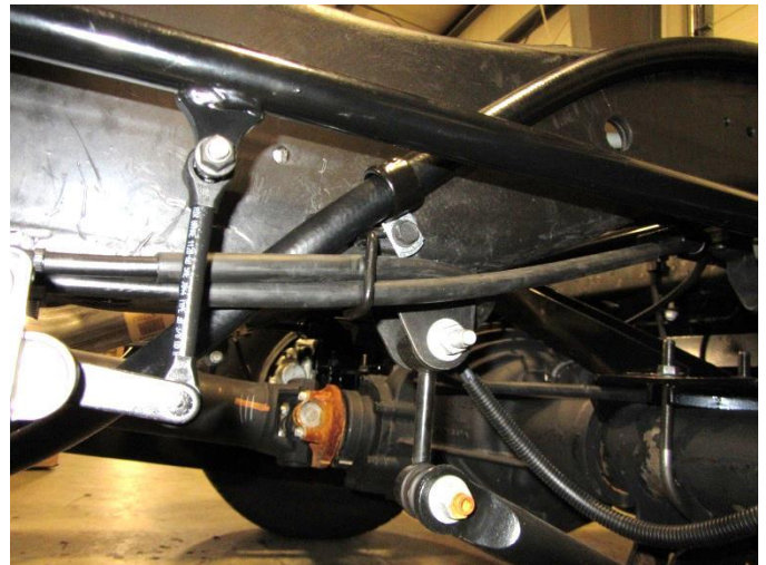
Figure 57. Routing of parking brake cables.
