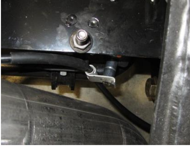
Figure 58. Passenger side parking brake remounting.
