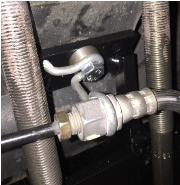
Figure 17. Brake Line Re-Attached to Lower Axle Clamp
