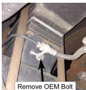
Figure 15. Remove Bolt from Axle Seat
