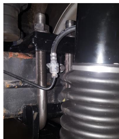
Figure 19. Attach OEM Bolts to Upper Axle Clamp Flange
