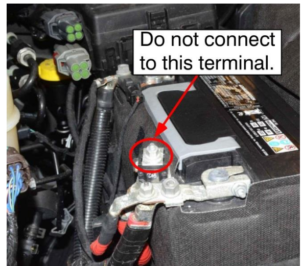
Figure 40. OEM Upfitter Driver Side Terminal Connection instruction.
