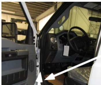
Figure 41. Accessing inside of side kick panel.
