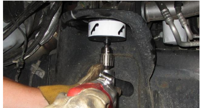
Figure 5: Cut a 4-1/2" hole around the OEM shock hole using a hole saw.
