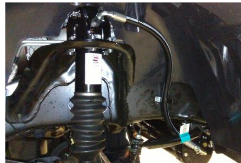
Figure 15: Hose routing from volume to strut
