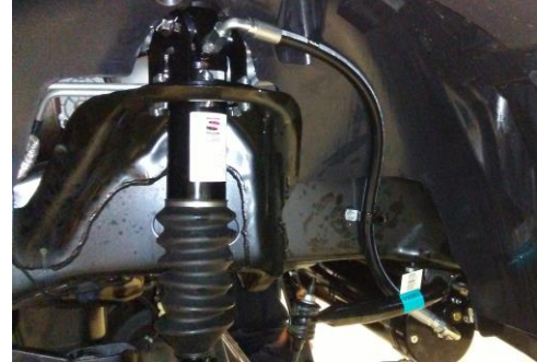
Figure 20: Hose routing from volume to strut. Note: FS70R configuration shown, FS73 similar.
