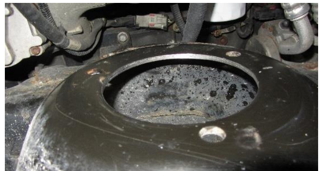
Figure 6: View of clean cut using hole saw.
