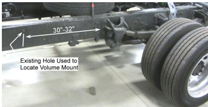
Figure 7: Locating Volume Mount to Frame
