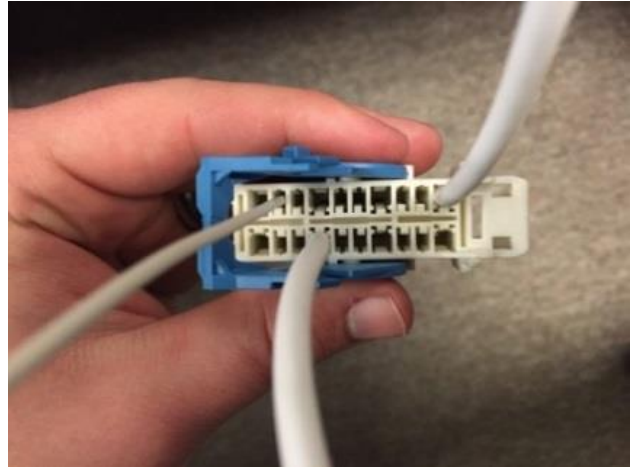
Figure 26: Three wires installed into service connector.
