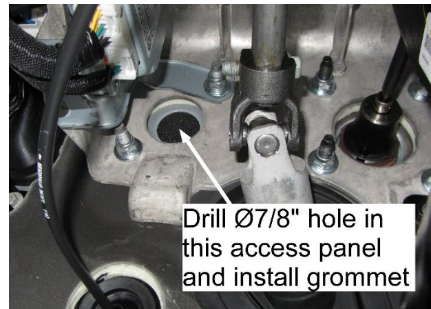
Figure 39: Cover plate to route harness through
