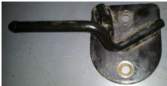
Figure 6: Enlarge holes to Ø17/32\"
