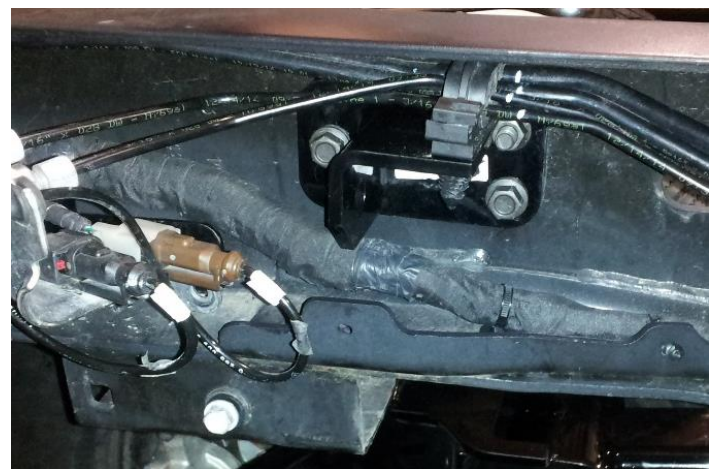
Figure 11: Tie Plate Bracket installed with fuel and brake lines reattached
