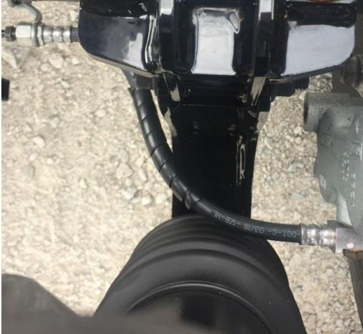
Figure 18. Spiral Wrap on Whip Hose
