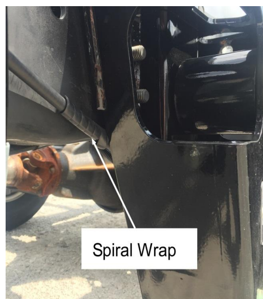
Figure 8. Spiral Wrap Around E-Brake Cable
