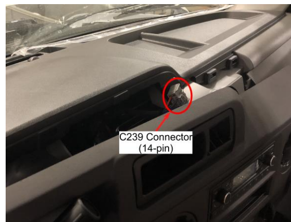
Figure 38. C239 Connector Location
