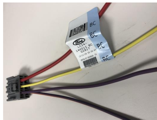
Figure 34. C215 Upfitter Connector
