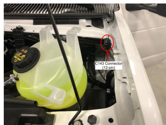
Figure 35. Locate C143 Connector
