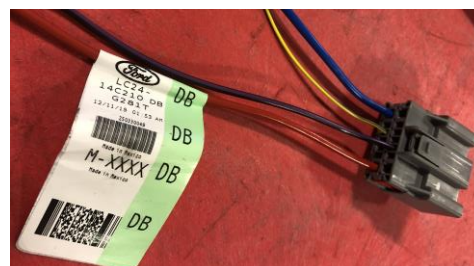
Figure 39. C239 Upfitter Connector
