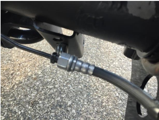
Figure 19: Use Spacer Tube & M8 Bolt to Re-attach Bracket
