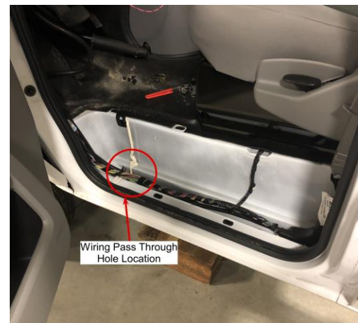
Figure 32. Location of Driver Side Access Hole
