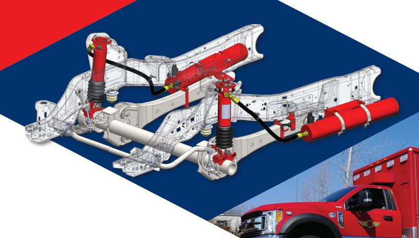
• Integrated with LS CLASS® rear drive axle suspension
