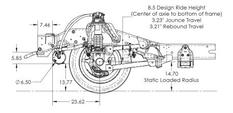
Discover the next generation suspension system designed specifically for light and medium-duty truck applications for producing a smoother, luxury-style ride.
