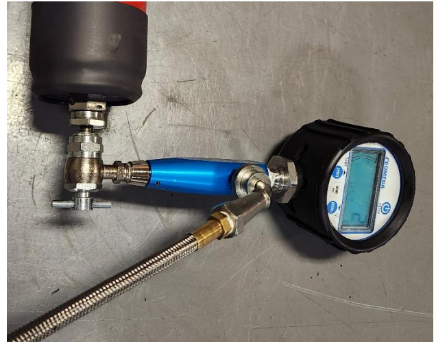
Figure 7. Fill hose attached to Fill Tool.
