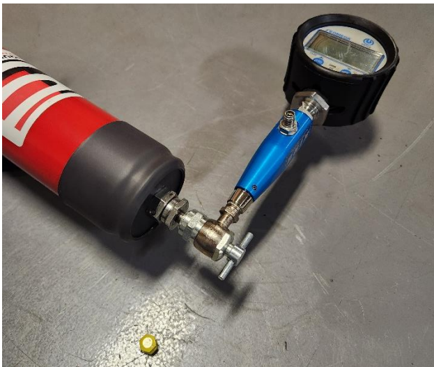
Figure 6. Fill Tool attached to Accumulator
