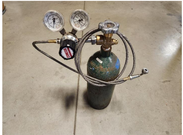
Figure 4. Example of Fill Station
