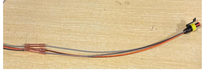
Figure 7: Butt Spliced New Harness
